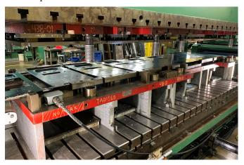
Second, we designed and built a progressive die to support this new onepiece design. Throughout the prototyping we utilized our fiber laser to cut different strip configurations and fine tune the die design to eliminate wrinkles.
