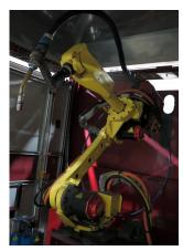
And with two robotic welders, the CNC Panasonic Robotic Welder and the Genesis Robotic Welder, Ultra can produce two footboards at a time – decreasing downtimes and increasing production rates.
