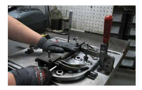
A customized functional gage designed and built by Ultra tested the placement of the welded hinges ensuring the footboard was ready for assembly.
