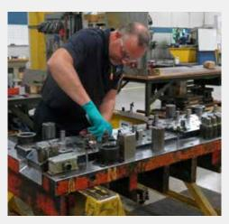
This manufacturer of metal components for security systems was finding it difficult to perform scheduled preventative maintenance on its stamping dies for two main reasons.
